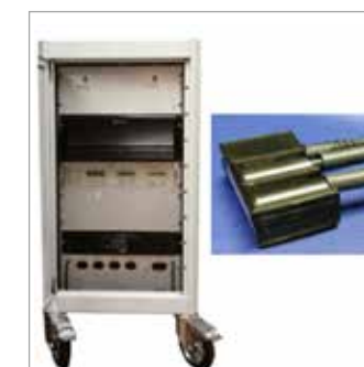
Fig. 1 - In-house built TD-fNIRS medical device and custom 3D printed probe for skeletal muscle measurements.characterization using FROG.
