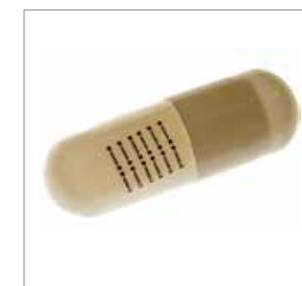
Fig. 1 - Photograph of an array of organic transistors transferred on a commercial pharmaceutical capsule by means of tattoo-paper transfer.
