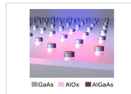
Fig. 2 - Sketch of the studied Al_{0.18}Ga_{0.82}As -on- AlOx platform. It consists of a GaAs wafer with Al_{0.18}Ga_{0.82}As cylinders on top of a 1- \mu m -thick aluminum oxide (AlOx) layer. The resonators are 400 nm high, with radii varying between 180 nm and 220 nm, placed at a distance of 3 \mu m from each other
