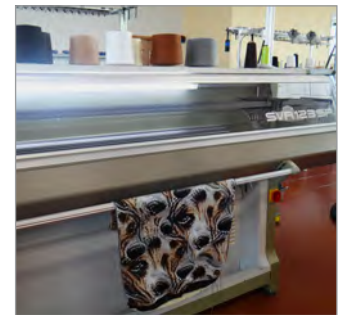
Fig. 2 - Jacquard fabric produced by the Shima Seiki knitting machine. Maglificio Pozzebon. Photo by A. Alves Santos.
