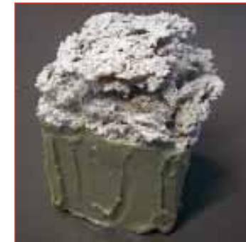
2. Salt-induced damage of a mortar specimen
