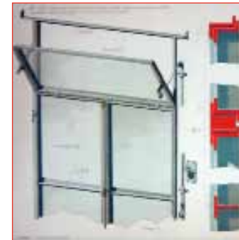
1. Iron window of commercial profiles (1909)
