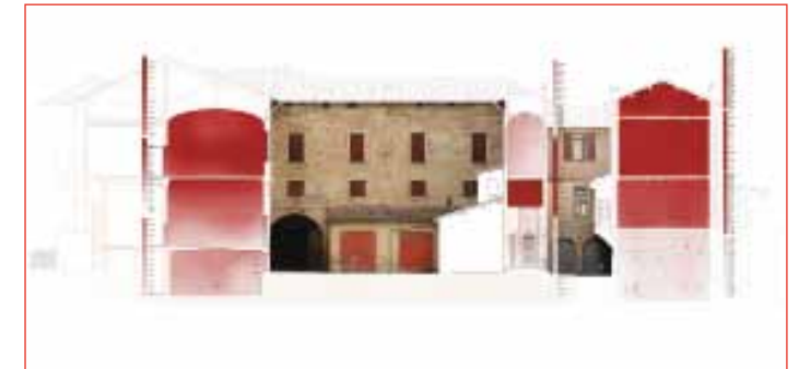
3. The monitoring of the microclimate. Distribution of temperature in the longitudinal section of the Rocca Rangoni in Spilamberto (MO)
