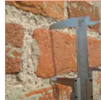
1. Measure of brick thickness by calibre
