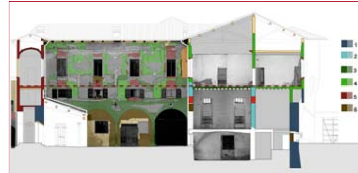
3. The Rangoni fortress. Courtyard section with the indication of transformation phases; in red the noble level of the "vago palazzo" (phase 5: 1641-1660) built restoring the previous disposition of the rocca (phases 1-5)
