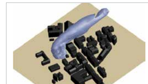
Hazardous gas dispersion simulation from an industrial accident
