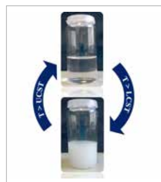
Fig. 1 - Visualization of the phase transition for polymers with a LCST or a UCST behaviour.
