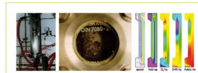
5. Lab-scale air-lift gas-liquid reactor and simulation of flow field, gas hold up and concentrations of main reactants (cyclohexane oxidation to adipic aci.).
