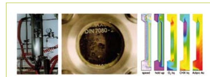
5. Lab-scale air-lift gas-liquid reactor and simulation of flow field, gas hold up and concentrations of main reactants (cyclohexane oxidation to adipic acid)
