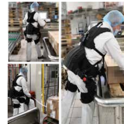
Fig. 2 Images from one of the field test in food processing plant. The OE was used in the warehouse section of the company. The custom surveys collected subjective effects regarding physical ergonomic of our XoTrunk.
