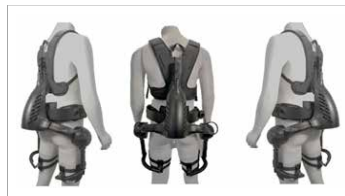
Fig. 1 - The XoTrunk is an active back-support exoskeleton designed to reduce lumbar loading on users performing manual material handling activities. It is a rigid exoskeleton that weighs approximately 6 kg and is powered by an onboard battery. Two electric actuators are aligned with the hip joints axes of flexion-extension and generate the assistive torques in the sagittal plane to support hip and back extension. The assistive torques are transmitted to the wearer as assistive forces applied onto his/her torso and thighs, through the body attachments.
