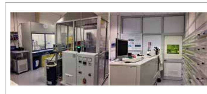
Fig. 1 - Overview of nitinol prototyping laboratory. On the left: salt bath equipment and fluidized bed for shape setting (thermal treatment), chemical etching and electropolishing equipment under chemical hood for post-processing and surface finishing treatments. On the right: Nd:YAG laser cutting equipment with nitinol tube availability.
