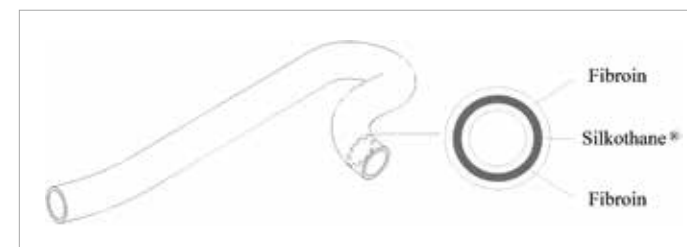
Fig. 2 - Silkothane ® graft and respective cross-section depicting the three-layered structure.
