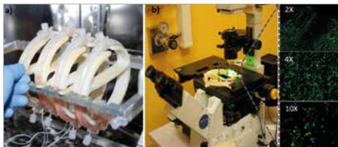
Fig. 1 - a) The bioreactor allows the release of a single culture chamber b) to perform the live imaging of labeled cells of the cardiac construct by means of a fluorescence microscope.
