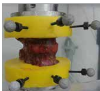
1. human thoracic functional spinal unit embedded in PMMA prior testing
