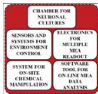
1. Scheme of the developed experimental platform intended for prolonged and parallel in vitro neuronal recordings by means of Microelectrode Arrays (MEA).
