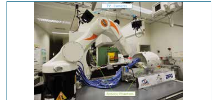
2. Experimental set-up at GSI. The beam line (solid red line), the robotic phantom and the optical tracking system TVCs are highlighted.
