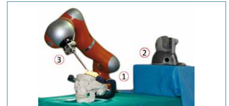
1. The robotic architecture: the robot (1) can be controlled through a master device (2) to perform an operation using a surgical tool (3)
