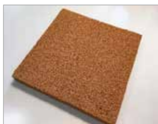
Fig. 1 – Sample of the investigated open-cell phenolic foam produced by Acell Industries LTD.
