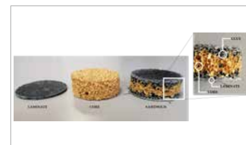
Fig. 4 – Sandwich materials samples. In the sandwich structure, the additional resin “layer” at the interface between each laminate and the core is visible.
