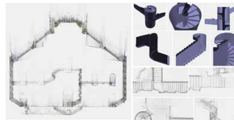
Fig. 3 Results of the 3D reconstruction of some narrow passages inside the Milan's Cathedral. Elevation view of the point cloud (left), plan view (bottom right) and 3D view of the mesh model (top right).
