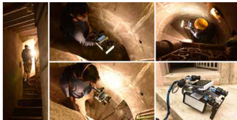
Fig. 1 Images of some narrow passages inside the Milan's Cathedral and of the first prototype of the proposed device employed during the survey operations.
