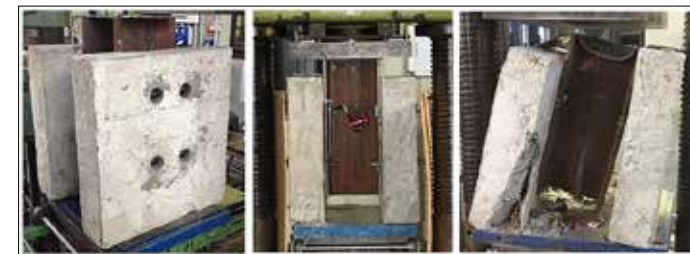
Fig. 2 - Specimen for push out tests (a), test layout in Material Testing Laboratory (LPM) of Politecnico di Milano (b), and failure of test specimen (c).
