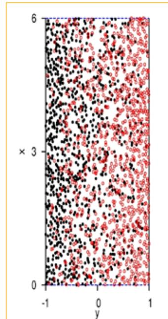
1. Steady state vortex configuration for case (a). Positive and negative vortices are respectively denoted by empty red and filled black circles.
