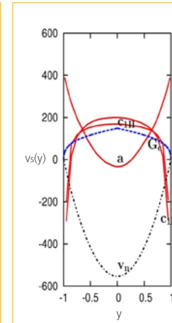
3. Coarse-grained superfluid velocity  $v_s$  for cases (a) and (c). The subscripts I and II indicate two different wall-nucleation distances for case (c).  $G_c$  is the analytical solution for case (c) and  $N_1=1876$ ,  $v_n$  is the normal fluid velocity profile.
