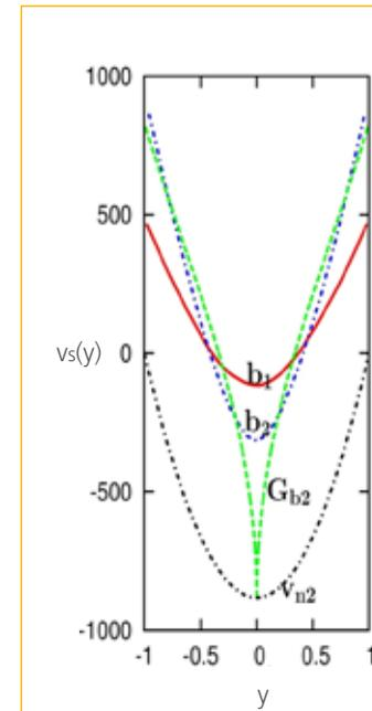
2. Coarse-grained superfluid velocity  $v_s$  for case (b). The subscripts 1 and 2 indicate respectively a number of vortices equal to  $N_1=1876$  and  $N_2=4800$ .  $G_{b2}$  is the analytical solution for  $N_2=4800$ ,  $v_n$  is the normal fluid velocity profile.
