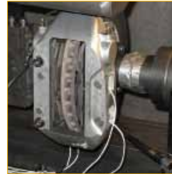
1. The brake caliper prototype under testing
