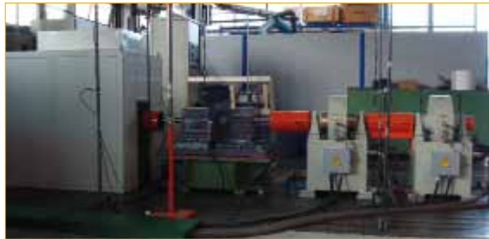
1. Test rig for the measurement of transmission error and noise of parallel axis gear sets
