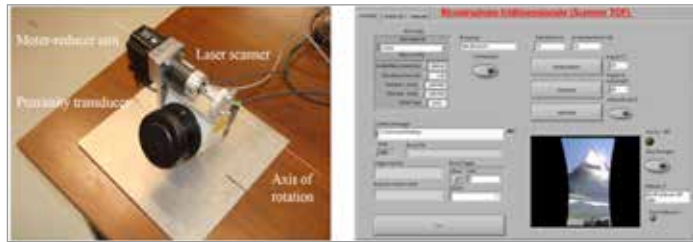
1. TOF acquisition unit: hardware components (left) and software control user interface (right).
