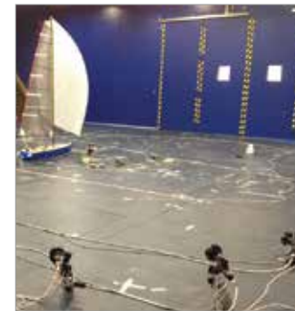
1. Wind tunnel sail shape measures with the stereoscopic system.
