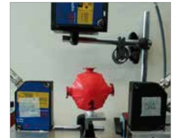
2. Experimental setup for measurement of displacement vs. pressure
