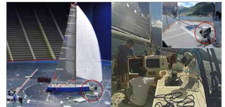
2. Wind tunnel and full scale sessions: disposition of the two laser scanners to detect the flying shape of mainsail and jib or gennaker.
