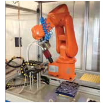
3. Robot bin-picking application using stereoscopy
