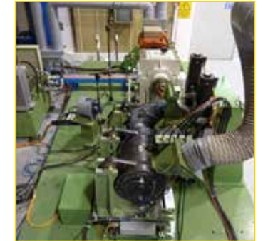
2. Test-rig for the diagnostic of rolling element bearings of a train traction system
