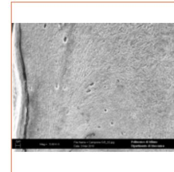
2. Cross-sectional SEM observation (500x) of a severely shot peened steel specimen
