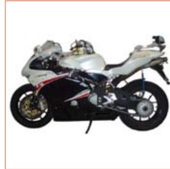
1. Instrumented motorcycle used during the experimental tests
