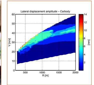
2. Map of the lateral motion amplitude of the carbody
