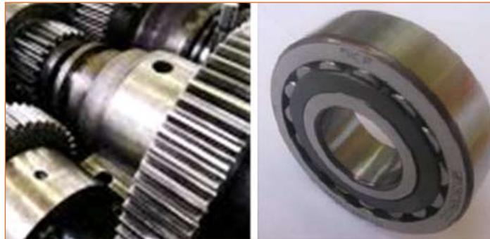
1. Rotating components considered in the research work: gearboxes (left) and rolling element bearings (right)
