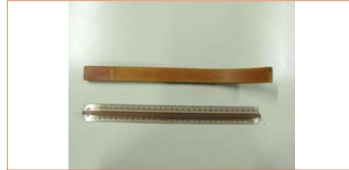
2. Prototype of collector lateral horn with thin SMA layers embedded
