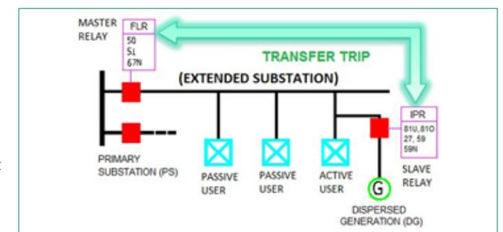
1. Interface protection relay with communication network.
