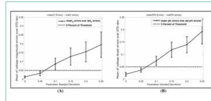
3. Ratio of the Mean of voltage magnitude errors (A) and voltage phase angles errors (B) by related Standard Deviations for IEEE 14-Bus test case. A horizontal dashed line is depicted to give an idea about the 5 percent of threshold, meaning that the state estimator is not biased for the network parameters uncertainty range below this line. According to the figures, it is apparent that the State Estimator is not biased for the parameters uncertainties up to nearly 7 percent.
