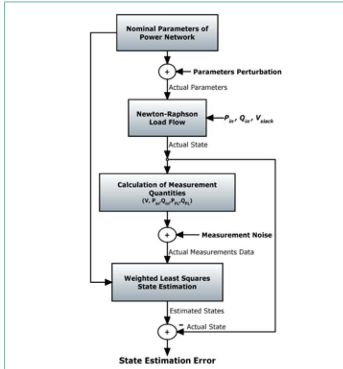
1. The flowchart of implementation. It is used in order to analyze the sensitivity of power system state estimation regarding to both the network parameters uncertainty and measurements uncertainty.
