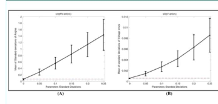
2. Mean and Standard Deviation of Voltage Magnitude Errors (A) and Voltage Phase Angle Errors (B) for IEEE 14-Bus test case. The figures clearly show that by growth of the network parameters uncertainty, the mean and standard deviation of errors considerably grows.
