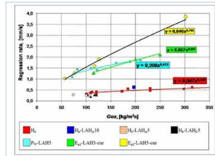
2. Regression rate of two epoxy-based fuels investigated in this study, compared with the best performance of the paraffin-based fuel (light blue) and the performance of the reference HTPB fuel (red curve).
