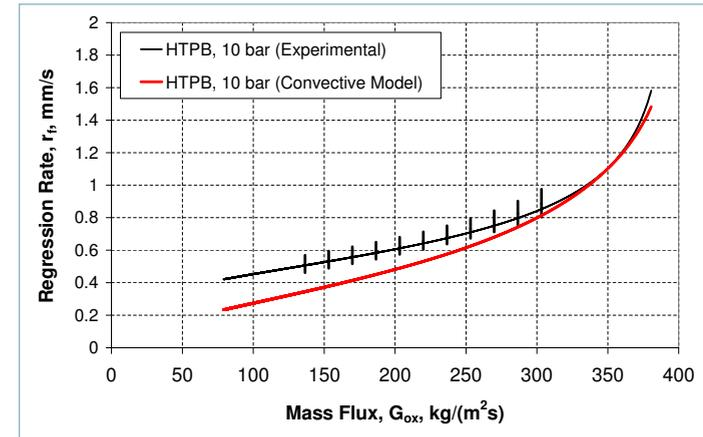
1. HTPB burning under  $G_{ox}$  with chamber pressure of 10 bar, comparison of experimental data and convective model evaluation. Note high agreement between experimental and numerical data for  $G_{ox}$  higher than 250 kg/(m<sup>2</sup>s). Differences in  $r_f$  for lower  $G_{ox}$  values mainly due to radiation effects.
