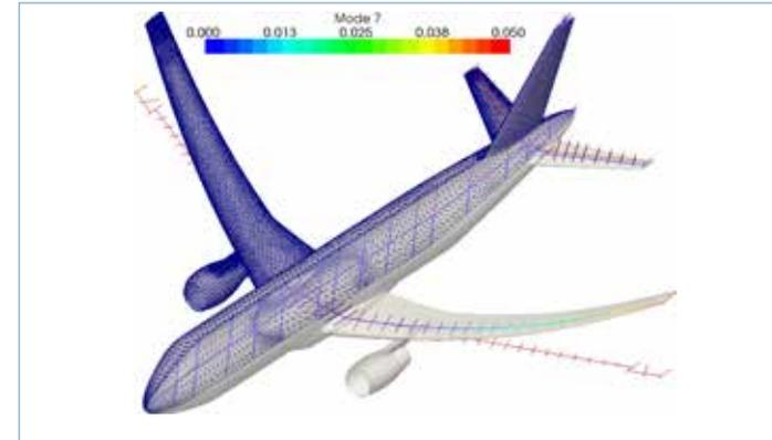
2. Aeroelastic interface and aerodynamic mesh deformation.
