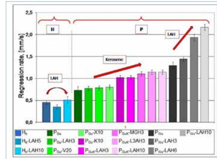
1. Regression rates of paraffin-based fuels added with different metal hydrides investigated in this study. Oxygen mass flux:  $G_{ox} = 120 \text{ kg/m}^2 \text{ s}$ .
