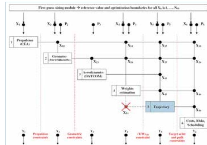
2. DSM for conceptual ELVs design: analysis proceeds sequentially from left to right along the diagonal, with terms above/below diagonal representing feed-forward/backward information flows.
