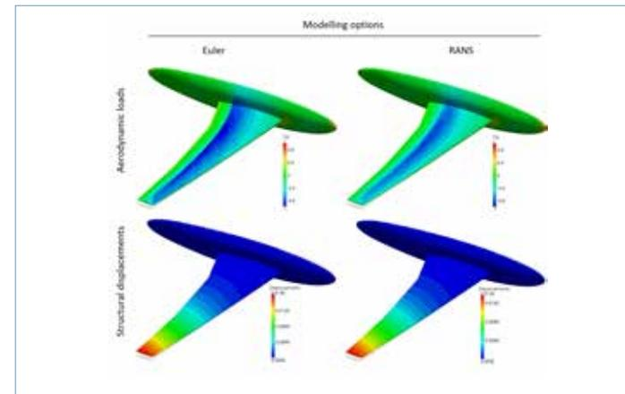
3. Aerodynamic loads and structural displacements for the static aeroelastic analysis of the HiReNASD wing as a function of modeling options (Euler vs. RANS).
